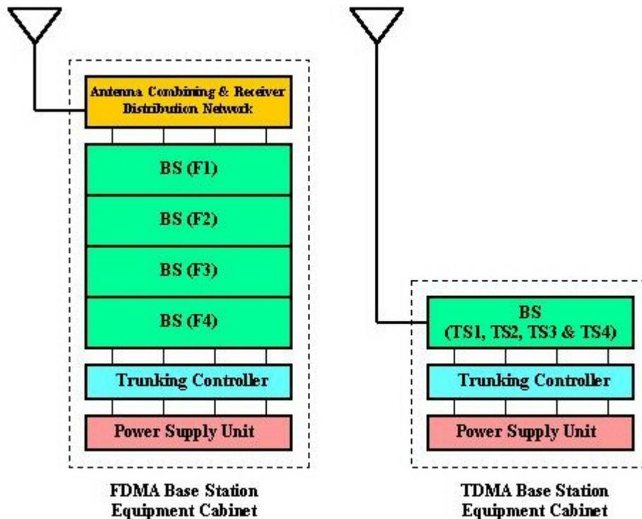
**Figure 2: Typical FDMA and TDMA 4 Channel COMPREP Configuration**
