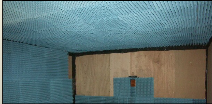
In addition to the metallic fabric, the testing room has been fitted with a pyramid shaped absorber which adds extra shielding and allows us to create a uniform electromagnetic field in the testing area.
