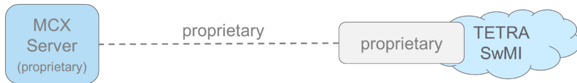
Figure 6: Proprietary interworking functionality MCX (implementation option 4)
