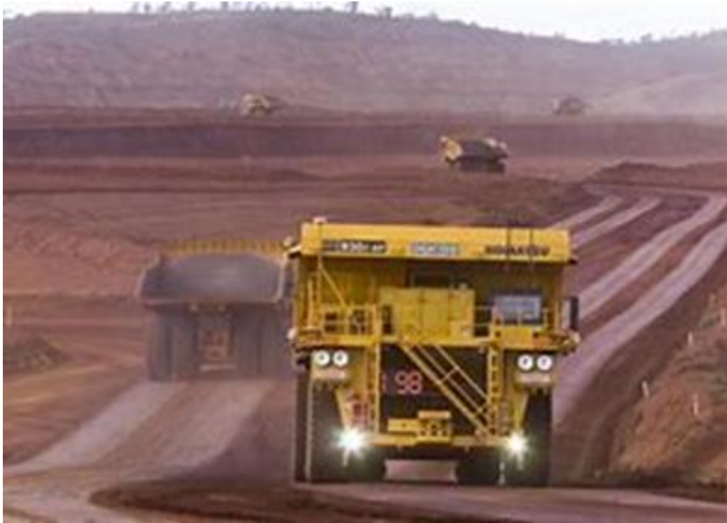
Autonomous mining haul truck using 4G/5G networks
