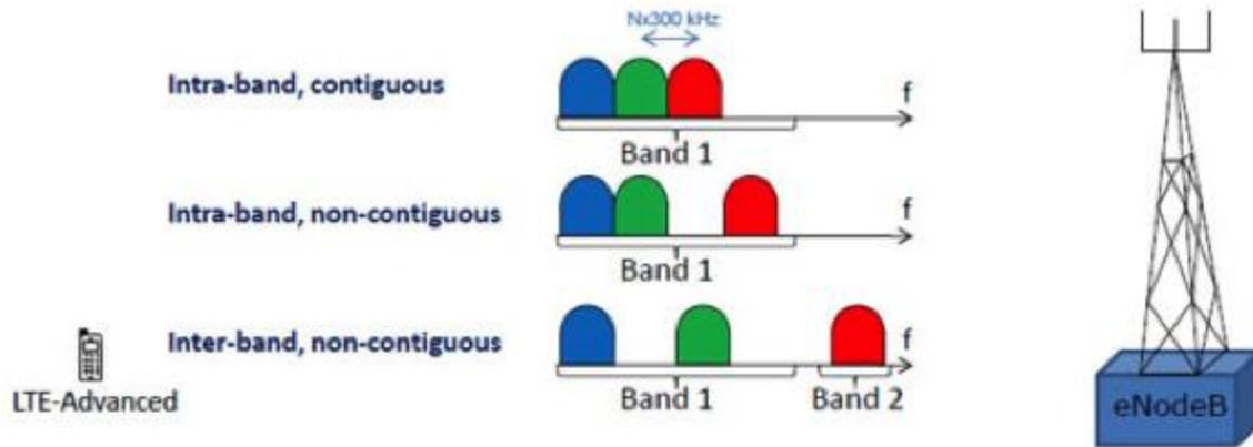
**Figure 6: Carrier Aggregation intra-band and inter-band aggregation alternatives**
